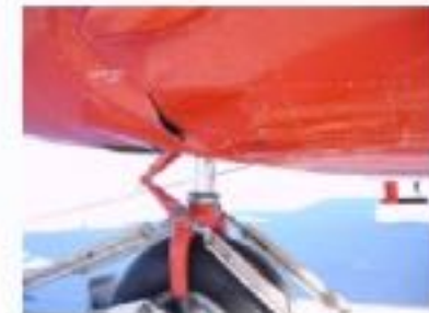
Buckled landing gear
